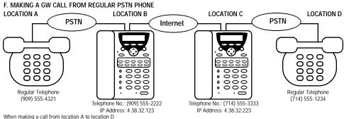
VoIP Phone at Location B must set GW enabled and set up VoIP Phone at Location C to it's shortcut dial between  $\pm$  1- $\pm$ 5
